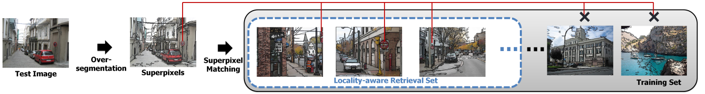
Fig. 2. The process to extract the retrieval set by super-pixel matching. The test image is first oversegmented into super-pixels. Then, we compute the similarity between the test image and each training image as described in Algorithm 1. (Please view in high 400% resolution).
